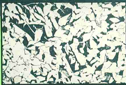
LARGER GRAIN OF ORIGINAL TUBING
