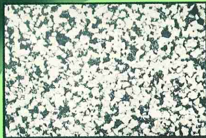
REFINED GRAIN OF LADISH FITTING
