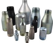
All of Westbrook's concentric and eccentric swages and bull plugs meet the requirements of ASME/ANSI B16.9 & MSS SP-95. Available from stock in Carbon Steel and Stainless Steel, our swage sizes range from 1/4" x 1/8" thru 8" x 2". Most reductions and schedules (S/10 through XXH), end preparations (TBE, PBE, PXT, BXT, BBE, & BXP). Bull plugs available 1/8" thru 8" in all schedules from STOCK. Also available in Chromes, Nickel Alloys & Exotics.
